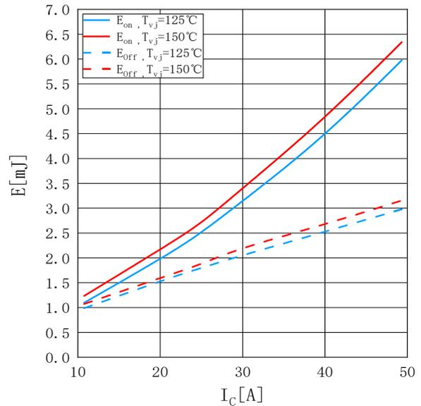
**Switching losses IGBT, Inverter (typical)**
