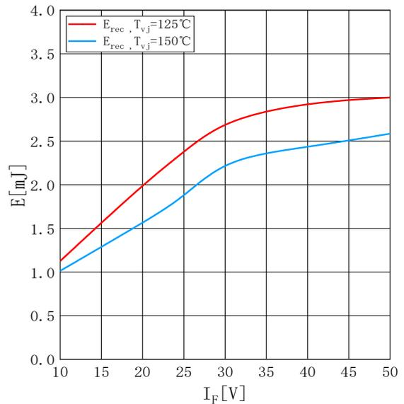
**Switching losses Diode, Inverter (typical)**
