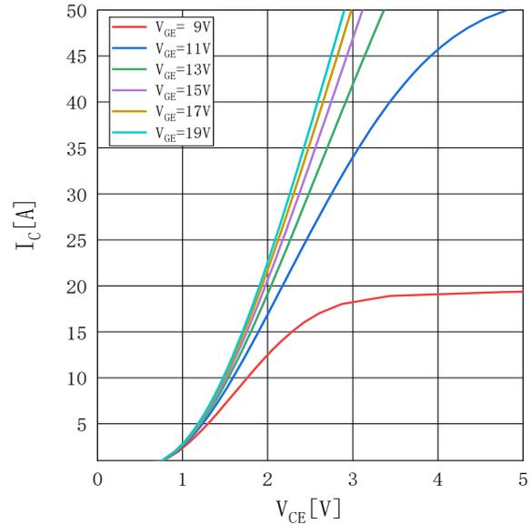
**Transfer characteristic IGBT, Inverter (typical)**
