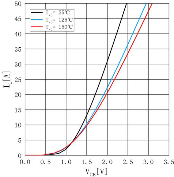
**Output characteristic IGBT, Inverter (typical)**
