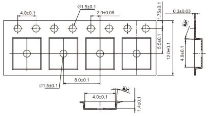
Cathode mark comes to reeding note side. The direction shall be one in a reel.
