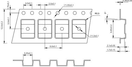
Cathode mark comes to feeding hole side. The direction shall be one in a reel.
