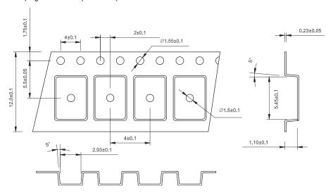
Cathode mark comes to feeding hole side. The direction shall be one in a reel.
