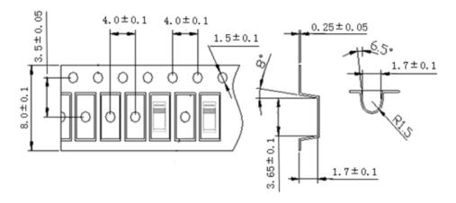
${f Notes}$  Cathode mark comes to feeding hole side. The direction shall be one in a reel.
